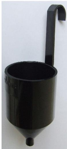
**Figura 5.** Viscosimetro a coppa di Ford con ugello da 4 mm: [https://en.wikipedia.org/wiki/Ford\\_viscosity\\_cup](https://en.wikipedia.org/wiki/Ford_viscosity_cup)
